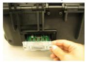
**6.** Tighten the screws on each side of the network module.
